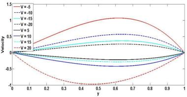
Figure 4.7: the influence of suction/injection on the velocity of the fluid.
