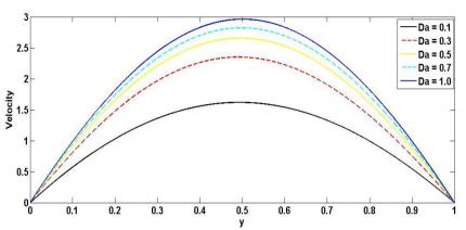
Figure 4.4: Velocity profile for  $\lambda = 100, V = 0.1, Pr = 0.71, Sc = 0.62, N = 0.01, Kr = 1.5$  with different values of Da
